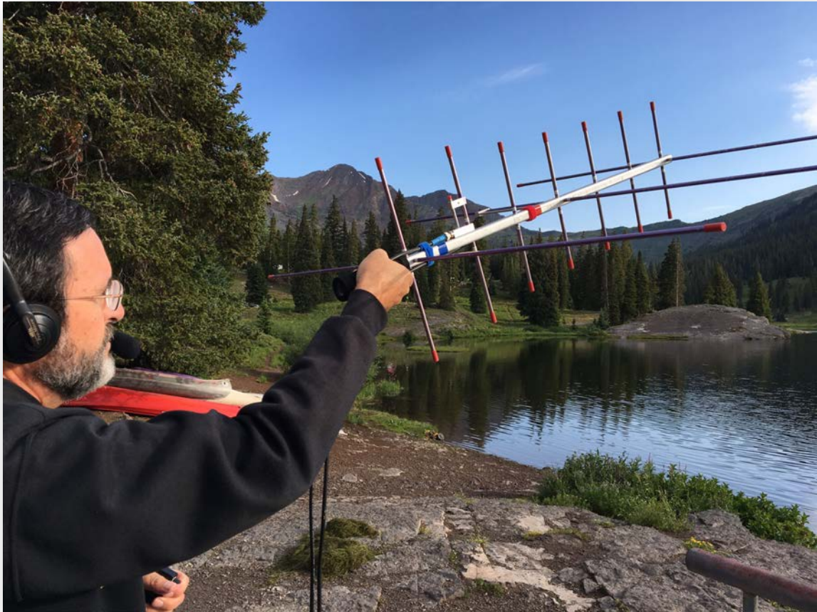
Steve, N9IP points his Arrow Antenna over Lake Irwin, Colorado. Note the use of red and blue tape on the boom and the coax to indicate VHF and UHF connections. He is wearing a Heil Pro Micro Dual iC headset and is using a Heil PTT Handswitch in his left hand. The radio was an Icom IC-821H, now replaced with an IC-9700.
